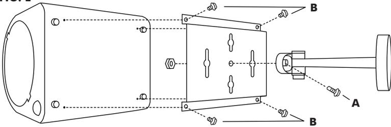
3. Attach the assembly to the wall: **FIG. F**
