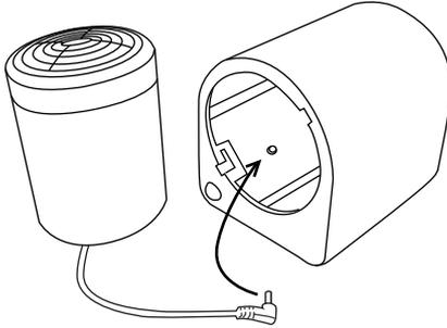
4. Insert the scent cartridge completely into the ScentWave™ by lining up the notches on the cartridge with the openings on the system. Lock by turning clockwise. **FIG. H**
